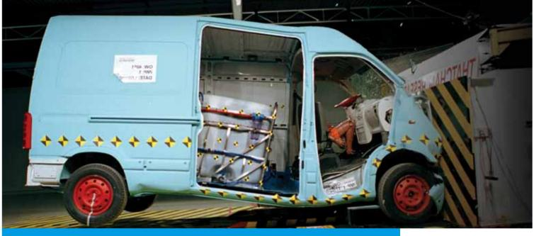
Uniquely, our van-mounted systems remain the only systems to have been tested to the international FMVSS-208 standard. In twenty years we are proud of our safety record in that none of our systems have become detached during a road traffic accident.
