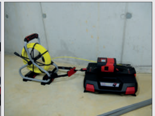
RM35 with Mounting plate- system case , Profi Set fiberglass rod Ø 4,5 mm
